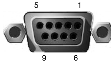
Fig 59. RS422 Connector as seen from the rear of the Multiviewer and Kahuna 360
