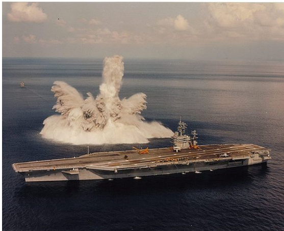
Shock test of Theodore Roosevelt during sea trials in 1987
