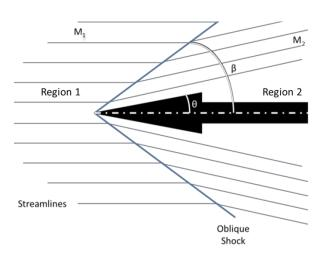
Figure 3: Schematic of an oblique shock.
