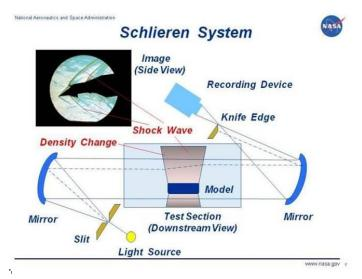
Figure 1: Schlieren system (Source: www.nasa.gov).
