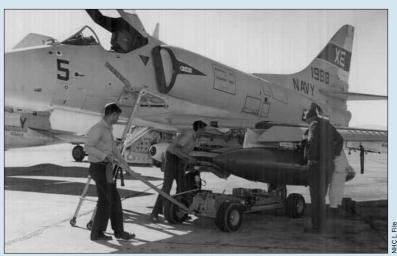
A Walleye being loaded on an A-4.
