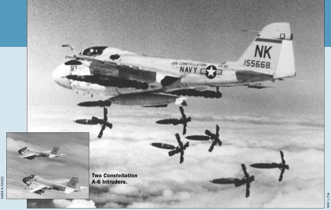
A Constellation A-6 Intruder drops a load of Snakeye bombs on targets in North Vietnam. The retarder tail of these bombs allowed low-level, high-precision attack while avoiding bomb-fragment damage to delivery aircraft.
