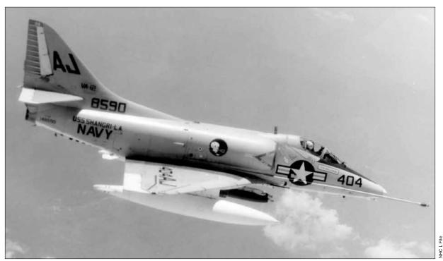
The Skyhawk, or "Scooter," as its pilots often called it, was designed in the early 1950s by the Douglas Aircraft Company with three goals in mind: it had to fly over 500 mph, carry a 2,000-pound bomb load to any target within a 460 mile radius, and cost less than \$1 million a piece.
