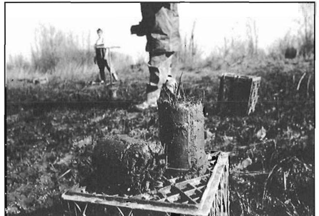
Figure 4. Golf-cup cutter transplant plug. Photo by M. Adams. GSC 2003-496
