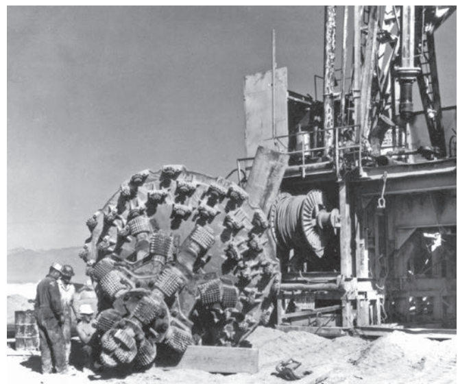
Drill bit for drilling a large nuclear test emplacement hole. Drilling time could require as much as 12 weeks of around-the-clock work, depending on the hole’s location, depth, and diameter. Large shots required a hole on average 1,000–2,000 feet deep and up to 12 feet in diameter. (Photo: Los Alamos)
