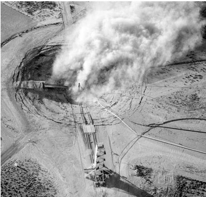
"Mandrel-Pliers," a nuclear test conducted in August 1969. The photo shows the surface around ground zero collapsing several minutes after the test, forming a subsidence crater 350 feet wide and 50 feet deep. (Photo: Los Alamos)
