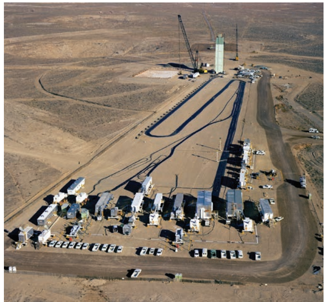
Preparations for the “Praetorian-Rousanne” nuclear test, 1981. The crane (background) is for lowering the nuclear device, along with a rack of diagnostic sensors for monitoring the explosion, into the test shaft. The trailers (foreground), stationed at a safe distance from ground zero, contain instruments to record the sensors’ diagnostic data, carried to the trailers by the miles of cables shown here snaking between them and the test. (Photo: Los Alamos)
