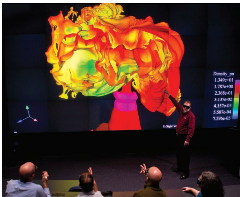
In lieu of testing nuclear weapons, second-generation designers judge the condition of the aging stockpile based on tests of weapon subsystems, computer simulations of both physics phenomena (shown here) and weapon behavior, and knowledge gained from past nuclear tests. (Photo: Los Alamos)
