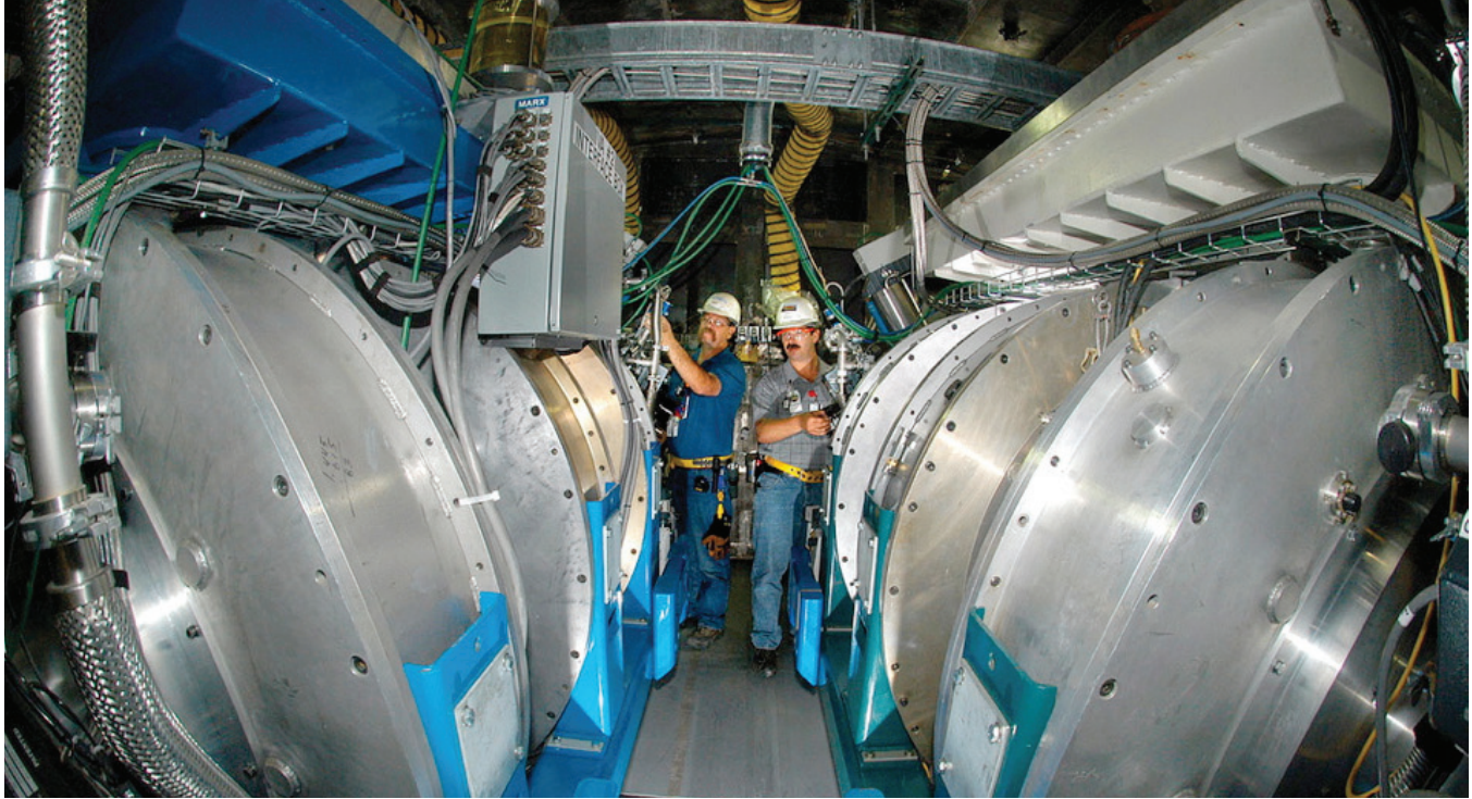
Highly trained technicians at the Nevada National Security Site maintain a high-intensity x-ray machine at the U1a experimental facility, built at the bottom of a shaft almost 1,000-feet deep. If approved, neutron-diagnosed subcritical experiments would be conducted at U1a. (Photo: National Nuclear Security Administration)
