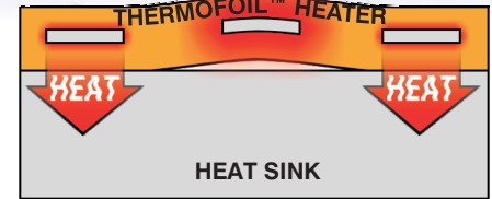
Voids or bubbles beneath the heater cause localized hot spots.
