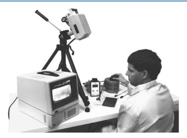
Typical heater test and prototyping setup: Heater (with multiple elements), variable power sources, digital temperature indicator, and infrared thermal imager.
