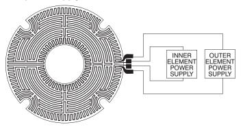
Custom dual-element heater for profile testing
